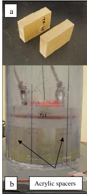
Figure 5.3. Acrylic spacers used for testing in air and water to hold top cap at the required height
